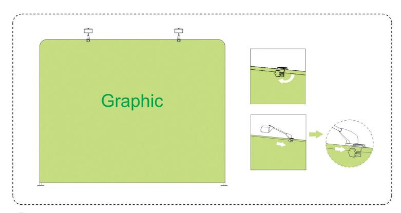
Out the light clip on the top of display and fix it with screw, then connect the light and the clip
